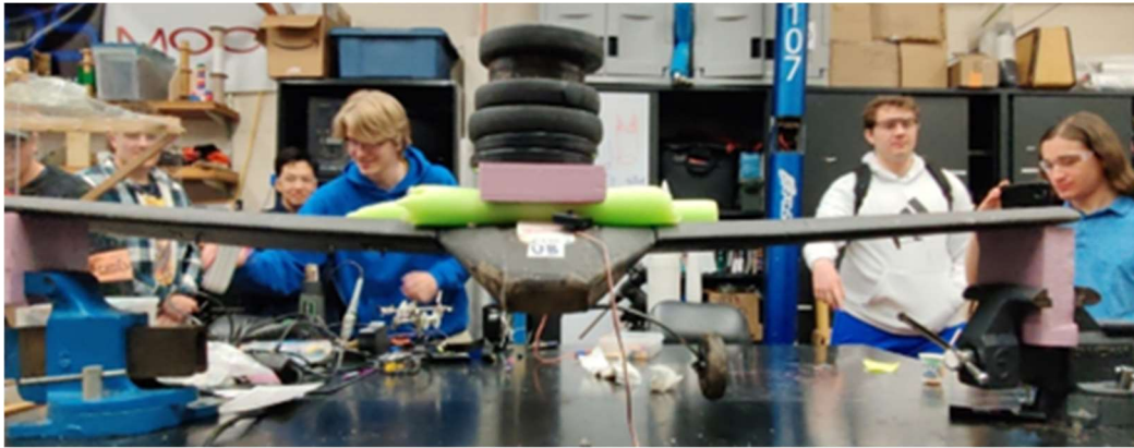
Figure 45. Wing structure test
