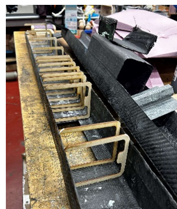
Figure 40. Fuselage with Ribs
