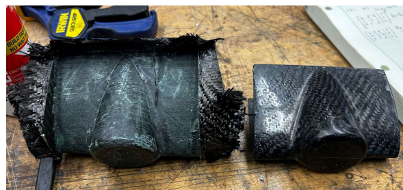
Figure 43. Nacelle Before and After Finishing
