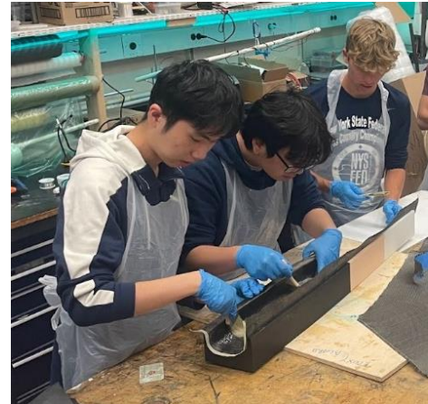
Figure 38. Fuselage Layup using 3D Printed Negative Molds
