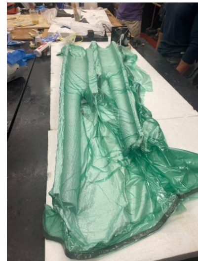
Figure 39. Fuselage in Vacuum Bag After Layup
