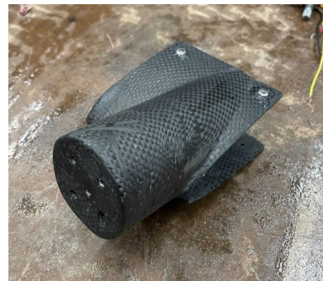
Figure 41. Nacelle After Finishing
